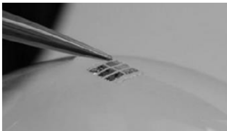
Figure 9. A flexible photovoltaic cell on a soap bubble, designed using large-scale polymer blend simulations.
