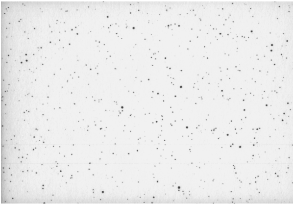
Figure 3. Sprayed droplets on a Syngenta water-sensitive card (52x76 mm) scanned using the DropVision.
