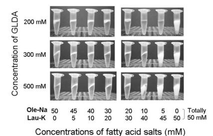
**Fig. 4.** Search for optimal ratio of Ole-Na over Lau-K for forming the hard layer of packed gels (discs of solid phase) collected over the media. Photographs show the gel layers formed and packed after centrifugation (14,000 rpm, 5 min).
