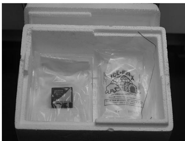
**Fig. 1.** Image of a data logger (left) and its position adjacent to an ice pack in a polystyrene foam container (right) prior to being enclosed inside a white single-walled cardboard box and shipped to designated locations in the USA.
