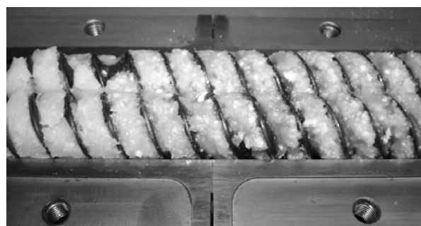
Fig. 1. Aggregated sodium caseinate in extruder barrel zone 5 and 6.
