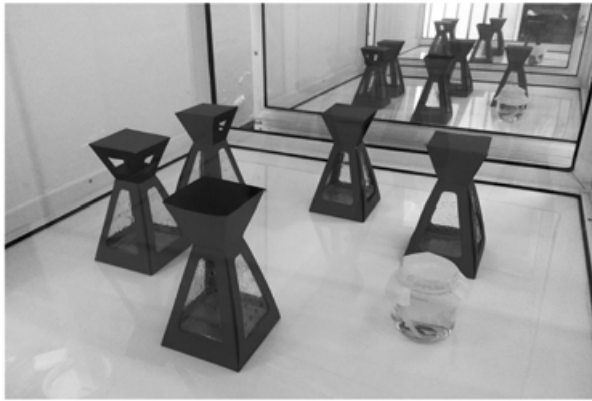
Fig. 2. Experimental setup to determine the response to trap entrances. Treatments include 1, 2, 3, 4 entrances and 1 wide entrance (4 replicas per treatment).
