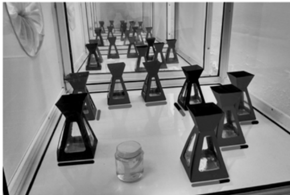
Fig. 3. Experimental setup to determine the response to color contrast. Treatments include red/black, orange/black, green/black and black/red and 4 control: red, orange, green and black (4 replicas per treatment).
