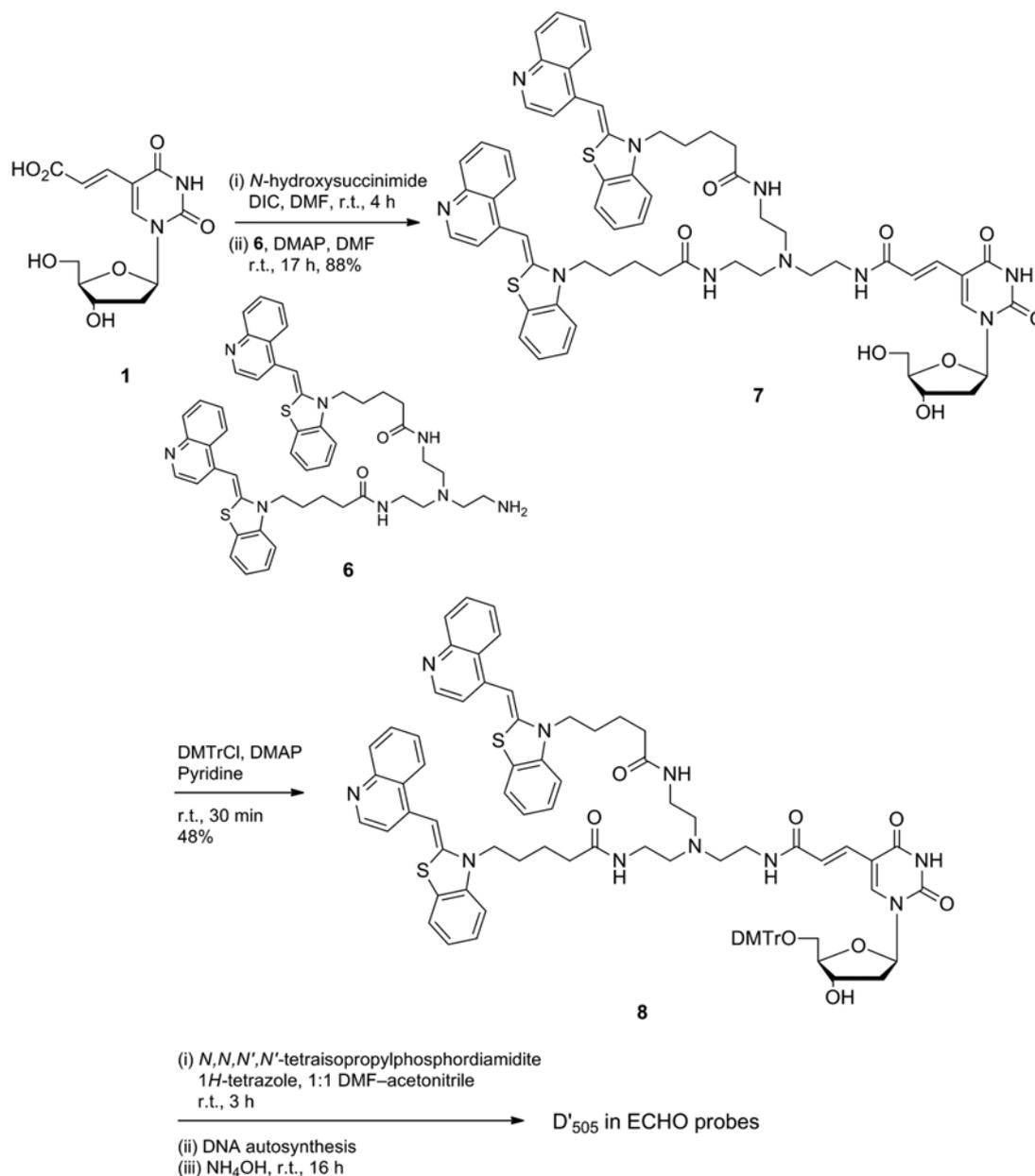
**Scheme 2.** Synthesis of **D'**<sub>505</sub>-containing ODN.
