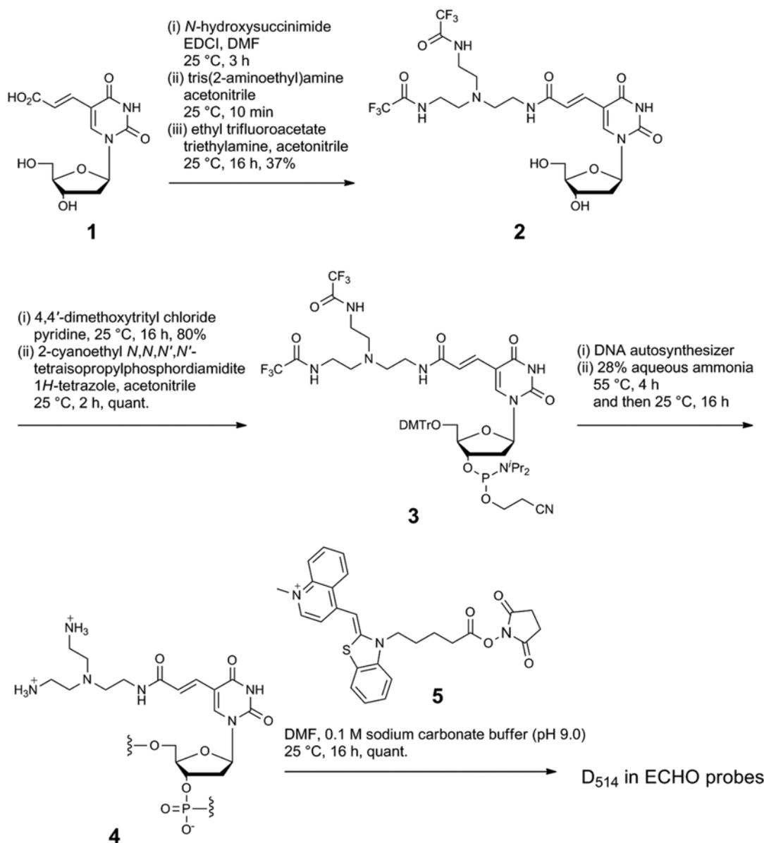
**Scheme 1.** Synthesis route of ECHO probes using a DNA autosynthesizer.
