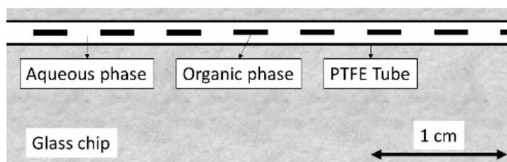
**Figure 3-5.** Picture of the slug flow in the microreactor. Picture adapted from ref. 84.
