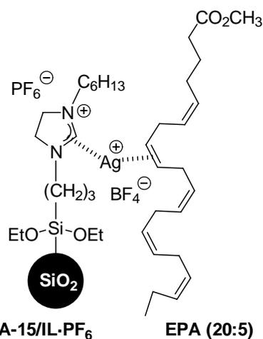
**Figure 3-6.** Schematic drawing of a silica-coated IL interacting with a PUFAME. Structure reprinted from Li, M., Pham, P. J., Pittman, C. U. and Li, T. 2009, *Microporous Mesoporous Mater.*, 117, 436 with permission from Elsevier..
