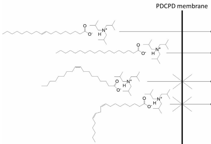
**Figure 3-18.** Graphic representation of FA separation using membranes. Adapted from ref. [122]
