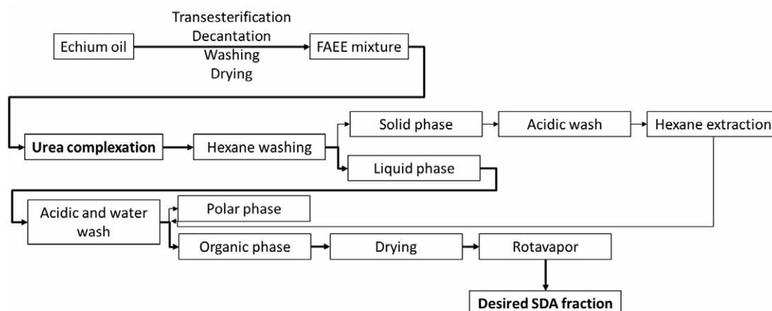
**Figure 3-3.** Example of a urea complexation flow chart for SDA purification using Echium oil. Information taken from ref. [76].
