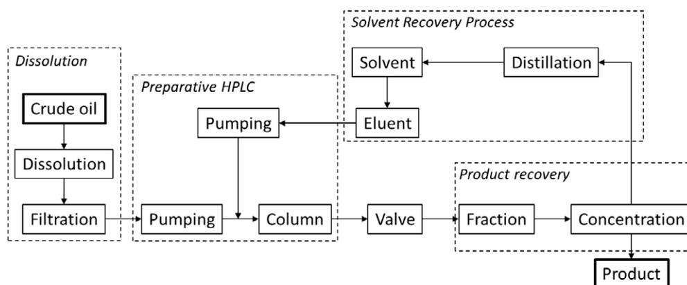
Figure 3-7. A flow diagram of the purification of DPA-EE and DHA-EE. Adapted from ref. [160].
