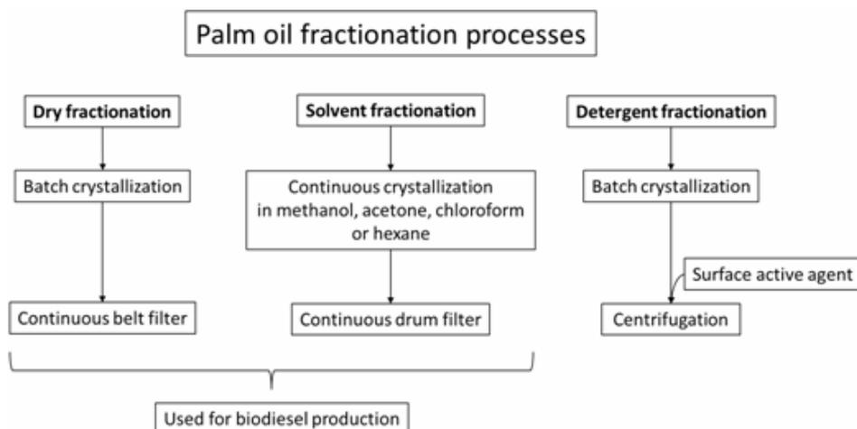
**Figure 3-1.** The three fractionation processes of palm oil that are applied in industry. Information taken from ref. [134].
