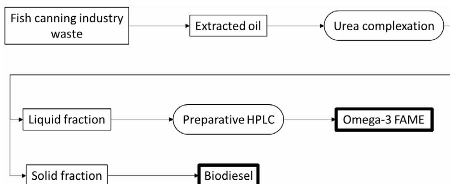
**Figure 3-19.** Example of a combination of different separation technologies for FAEE fractionation. Adapted from ref. [130]
