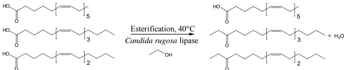
**Figure 3-11.** Example of a selective esterification for omega-3 purification using a lipase.
