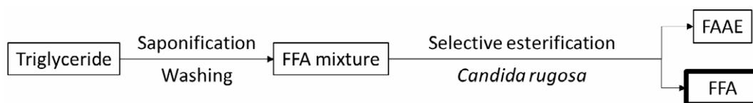
**Figure 3-12.** Example of a flow scheme using selective esterification for FA purification. In most research, the FFA fraction contains the desired FA compound.
