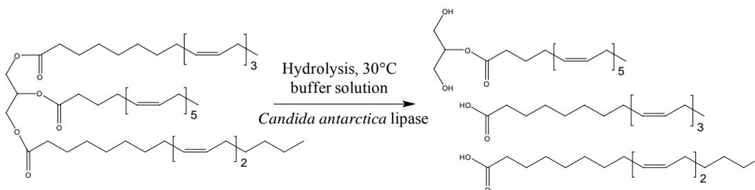
**Figure 3-10.** Example of a hydrolysis for omega-3 purification using a lipase.
