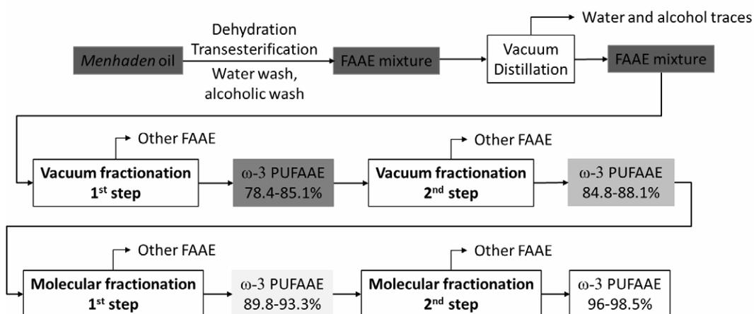
**Figure 3-4.** Example of a process for EPA and DHA concentration using vacuum and molecular distillation on pilot plant scale. Information taken from ref. [81].
