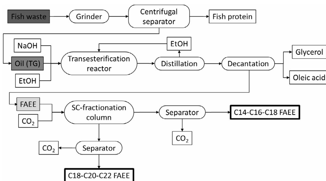
**Figure 3-9.** Simplified overview of the biorefinery concept for fish waste valorization. Scheme based on information from ref. [107].
