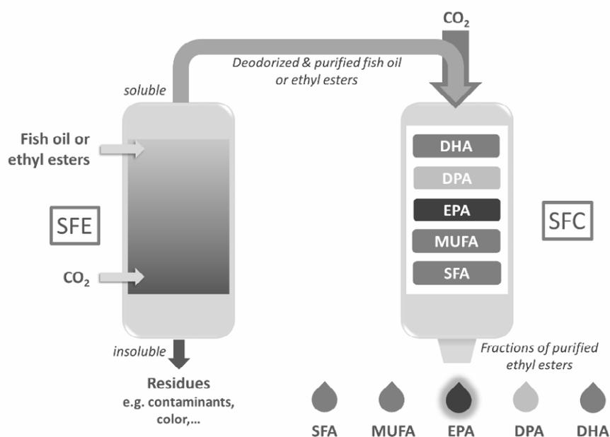
**Figure 3-8.** Graphic representation of the kd-pür<sup>®</sup> technology from KD Pharma. Adapted from ref. [174].
