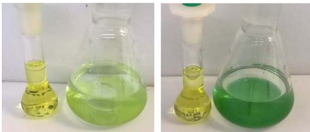
Figure 7. Left: A flask containing DcMeFc in DCB is mixed overnight in the beaker with the aqueous \text{CuSO}_4 solution. Pale green color indicates a partial oxidation of DcMeFc by atmospheric oxygen. Right: Adding LiTB in the aqueous phase turns yellow color immediately to dark green.
