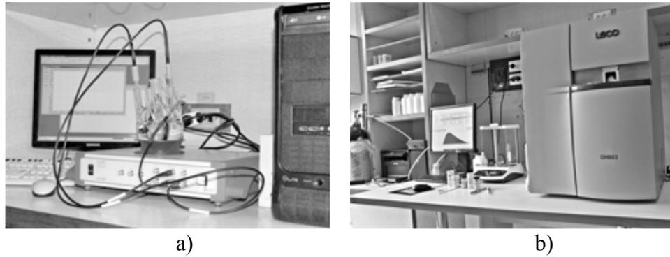
**Fig. 2.** Dynamic electrochemical laboratory VoltaLab40 (a) and hydrogen analyzer LECO DH603 (b).
