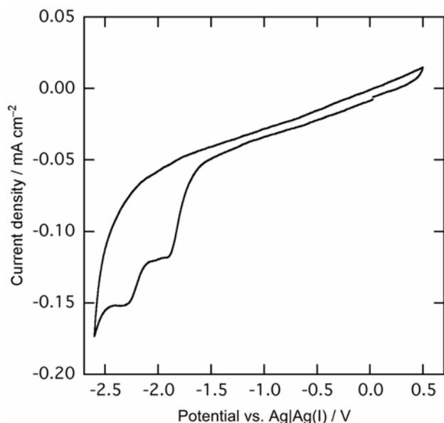
**Figure 1.** Cyclic voltammogram of a GC electrode in BMPTFSA containing 10 mM  $ZrCl_4$  at room temperature. Scan rate:  $50 \text{ mV s}^{-1}$ .
