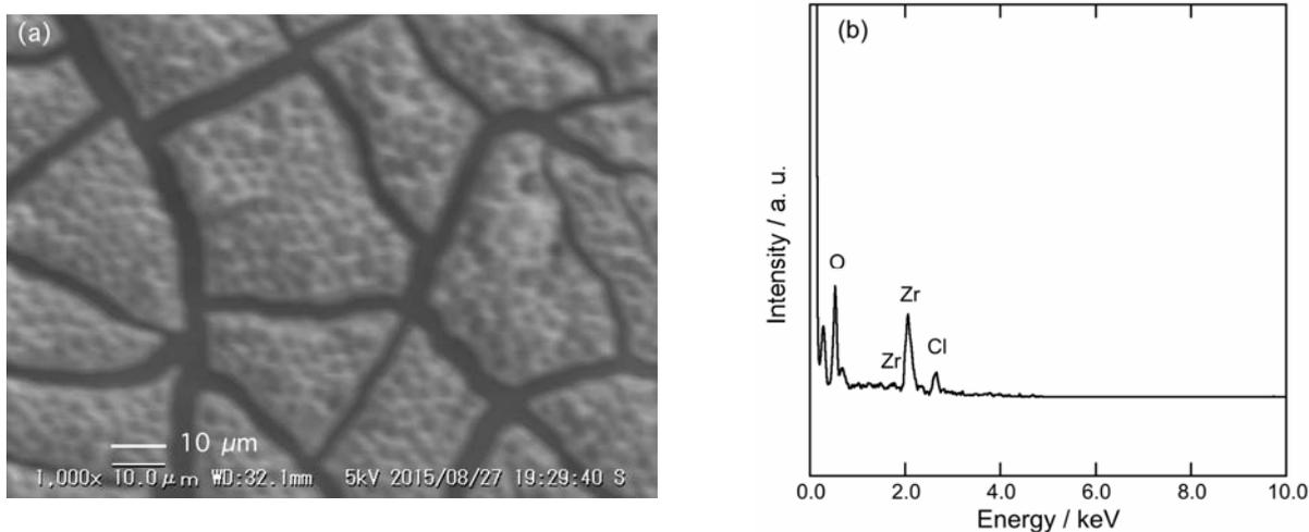
**Figure 2.** (a) SEM image and (b) EDX spectrum of the electrodeposits obtained on the GC substrate after electrolysis in BMPTFSA containing 10 mM  $\text{ZrCl}_4$  at  $-2.3$  V at room temperature.
