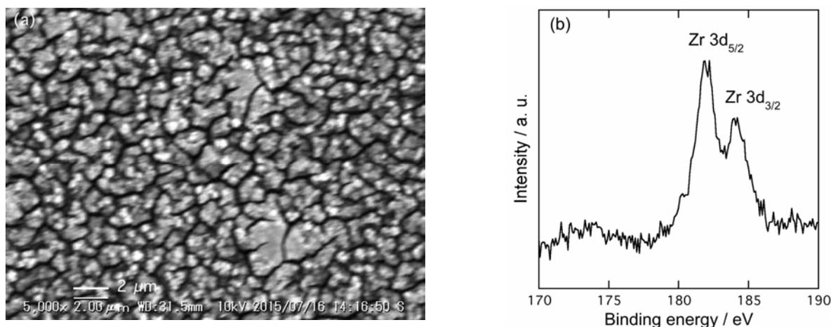
**Figure 4.** (a) SEM image and (b) XPS spectrum of the electrodeposits obtained on the GC substrate after electrolysis in BMPTFSA containing 10 mM  $ZrCl_4$  in the presence of 20 mM BMPCl at  $-2.35$  V. Temperature:  $100$  °C.
