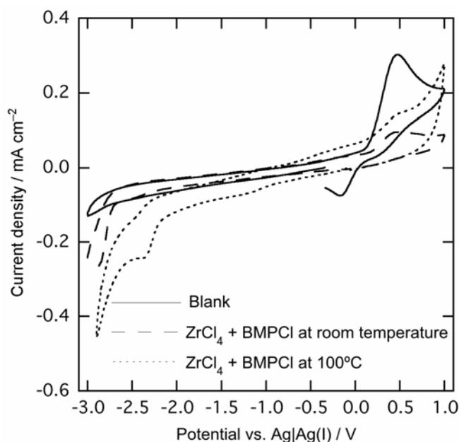
**Figure 3.** Cyclic voltammograms of a GC electrode in BMPTFSA containing 10 mM  $\text{ZrCl}_4$  with and without 20 mM BMPCl at room temperature and 100 °C. Scan rate:  $50 \text{ mV s}^{-1}$ .
