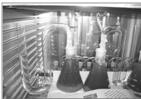
Figure 2. Anaerobic laboratory-scale bioreactor.
