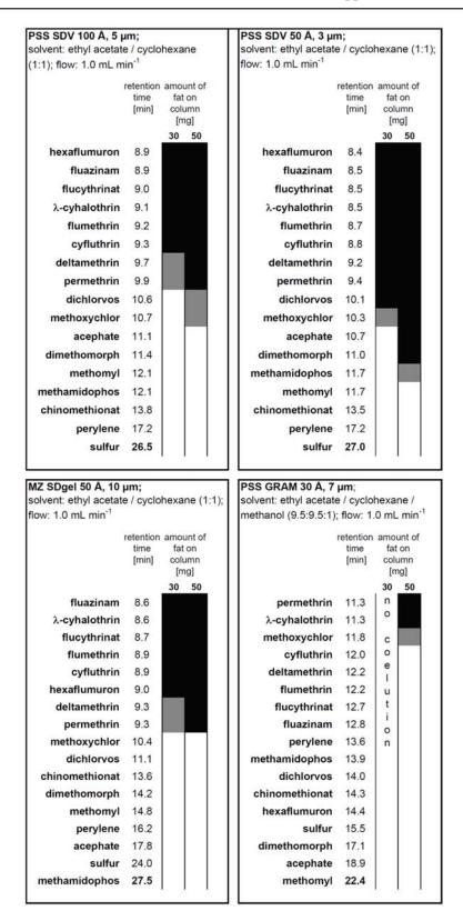
Figure 1. Elution profiles of four different analytical HR-GPC columns (8 mm x 300 mm) for selected pesticides and sunflower oil (black: full co-elution with sunflower oil; grey: partial co-elution with sunflower oil; white: no co-elution).
