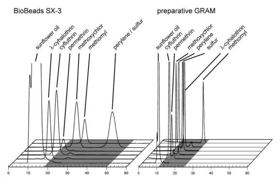
**Figure 2.** Separation of selected analytes from sunflower oil (400 mg on column) on BioBeads SX-3 column (flow 5 mL min<sup>-1</sup>; ethyl acetate/cyclohexane 1:1) and PSS GRAM column (flow 7.5 mL, ethyl acetate/cyclohexane/methanol, 9.5:9.5:1); grey areas: pesticide fraction (collecting period).
